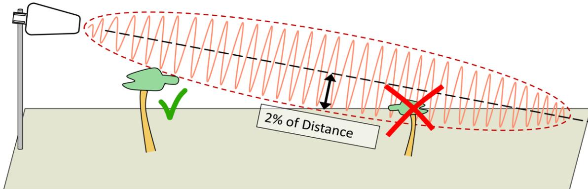
*The Line-of-Sight for a radio wave needs some clearance around the straight line.*
