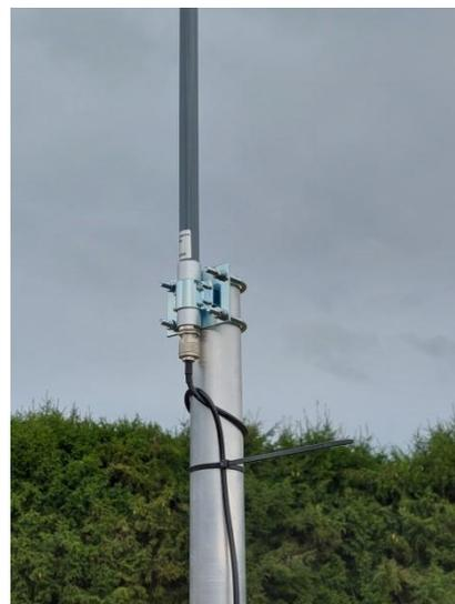
If you're using a short antenna cable, slip the Receiver onto the pole and tighten the backplate screws just a little. Add the Antenna to the pole. An omnidirectional antenna must sit on the highest end of it, having the highest U-bolt just 1 cm ( $\frac{1}{2}$  inch) below the top - otherwise the pole itself will interfere with the antenna and cause poor performance.
