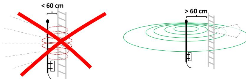
*Omni Directional antennas need at least 60 cm (2') clearance around the antenna. The same applies at all sides and the front of a Directive Antenna, but not behind it.*
